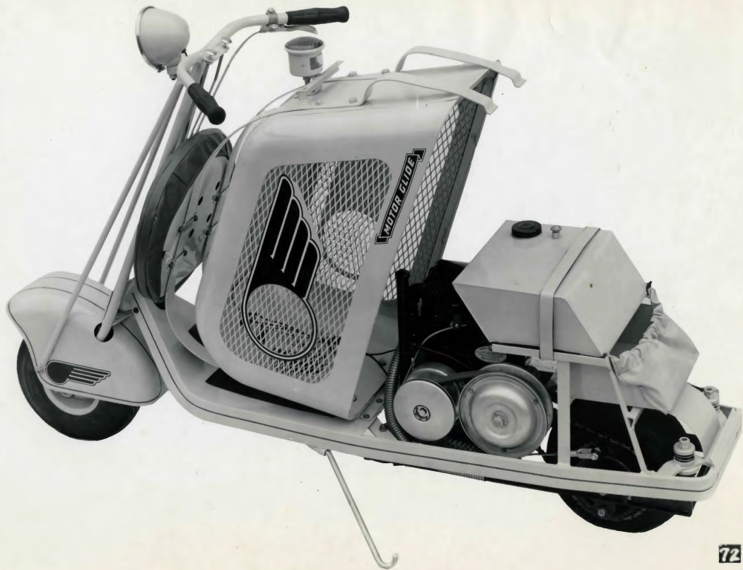
Salsbury Scooter Scrapbooks.com Ringed Hood in Forward Position, Showing Fuel Tank & Power Plant.
