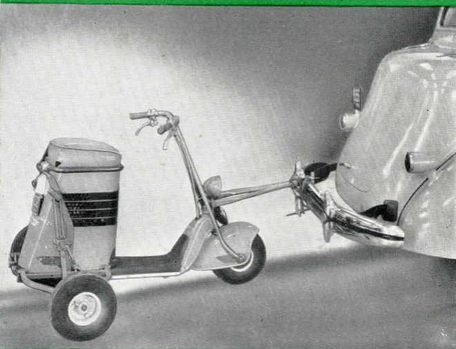
The cycle - tow for delivery and driver's return of automobiles.
